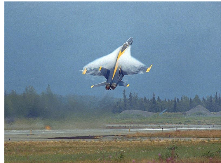
F-18: The impact on tail of the Leading Edge Extensions Vortex was reduced by wing strakes
